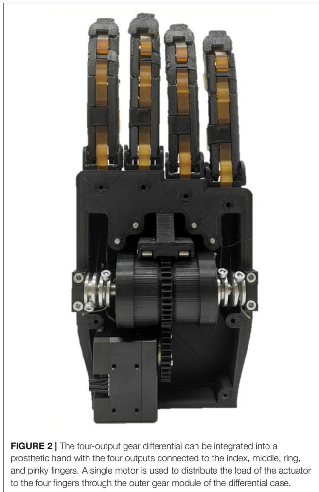
**FIGURE 2 |** The four-output gear differential can be integrated into a prosthetic hand with the four outputs connected to the index, middle, ring, and pinky fingers. A single motor is used to distribute the load of the actuator to the four fingers through the outer gear module of the differential case.
