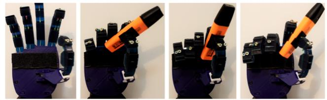
Fig. 10. The finger pivoting is responsible for the internal rotation of the highlighter pen. The proposed device has also the ability to re-orient objects within the hand.
